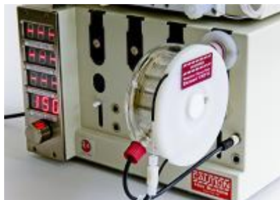
Standard PFA coil Ambient to 150°C
