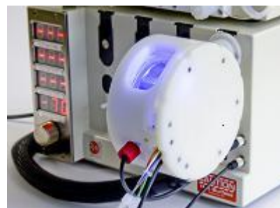
Cooled PFA coil Ambient to -70°C
