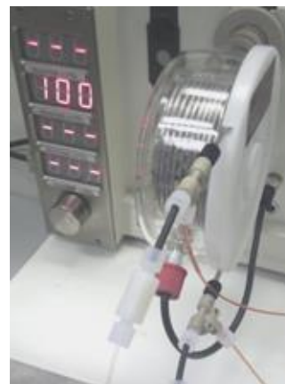
Gas/Liquid reactor Ambient to 150°C
