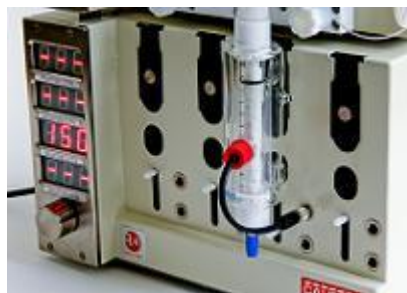
Standard Column Ambient to 150°C
