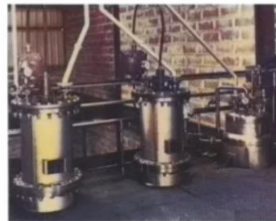
Pressurized Electrolysis Plant Developed by S.N.P.E. Research Centre
